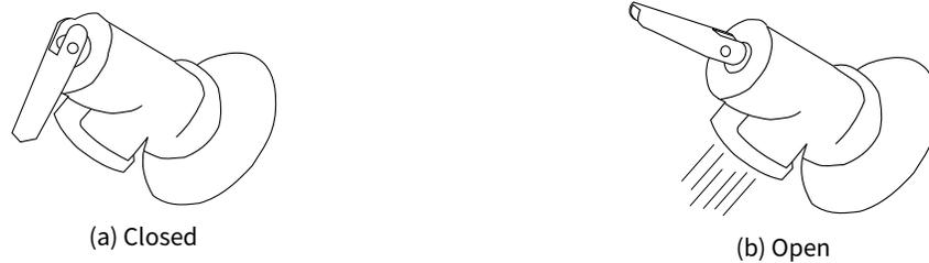
Close the pressure-release valve once water starts to come out. Turn off the water pump once it has stopped filling the hot water tank.
