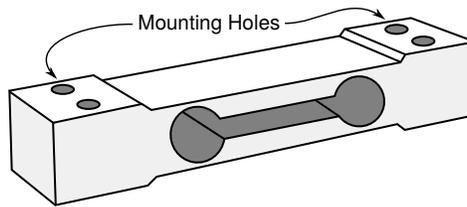
Figure 4: Load Beam Cell
