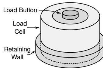
**Figure 2:** Button Load Cell
