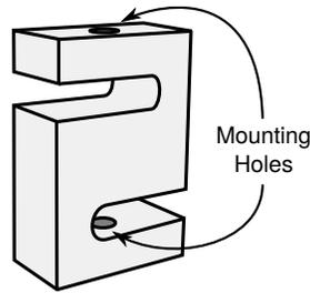
Figure 5: S-Type Load Cell
