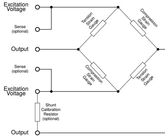
**Figure 7:** Basic arrangement of four strain gauges in a load cell
