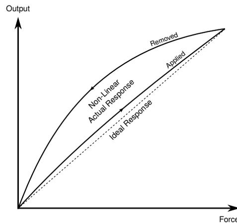
**Figure 8:** Non-linearity and hysteresis in a force-measurement system
