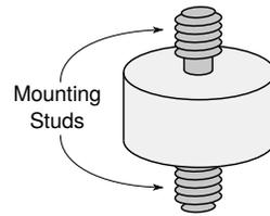
Figure 6: Rod-Type Load Cell
