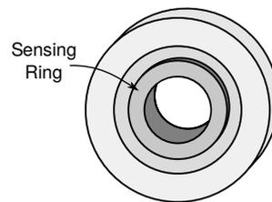
**Figure 3:** Thru-Hole/Ring Load Cell
