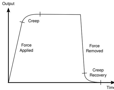
Figure 9: Creep curve of a typical force transducer
